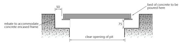
Due to the varying frame dimensions for different covers and decorative edging options, dimensions shown indicate the minimum amount of concrete required around the frame.
