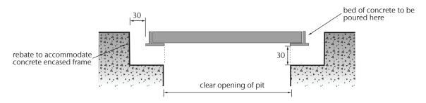
Due to the varying frame dimensions for different covers and decorative edging options, dimensions shown indicate the minimum amount of concrete required around the frame.
